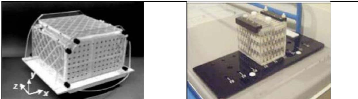
Fig.1 Linearity test object (LTO) developed at the Institute for Cancer Research. Fig.2 LEGO test object developed at the Institute for Cancer Research.
